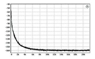
After applying passive RF interference filtering the results are already remarkable. Noise on 1kHz drops to –125dB, at 10kHz Noise comes even close to –160dB. But they improve even further when applying an active filter after the passive filtering.
